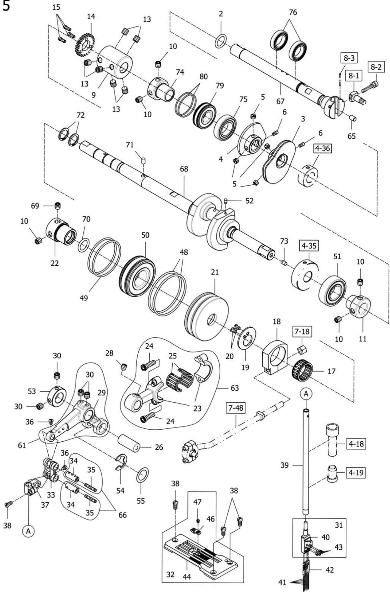
**MAIN SHAFT DRIVING MECHANISM**
