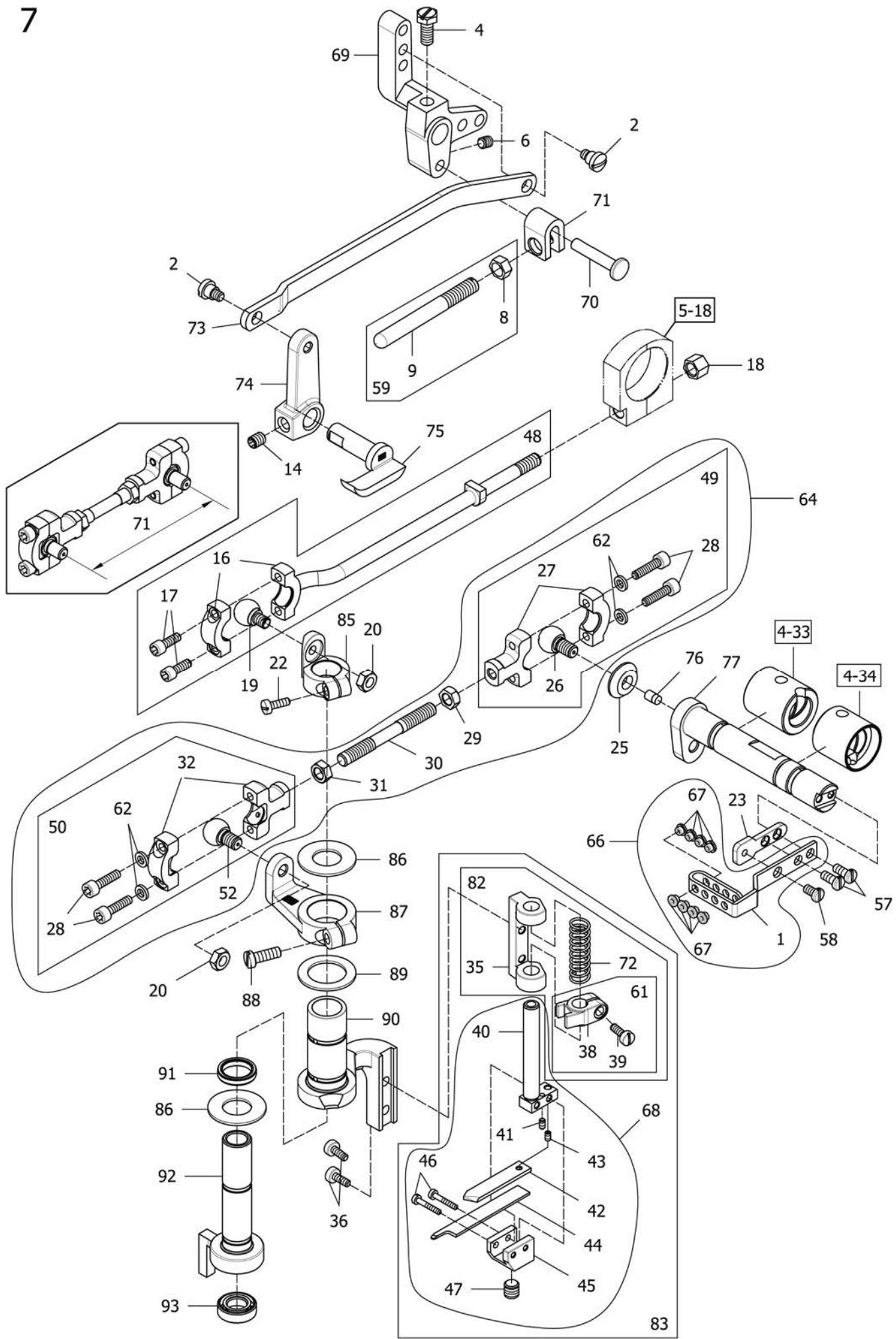
**UPPER KNIFE , CARRIER AND HOOK DRIVING MECHANISM 上切刀及上勾針驅動機構** 7
