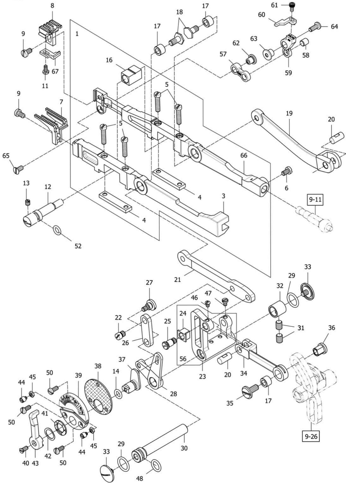
**FEED DRIVING MECHANISM**
