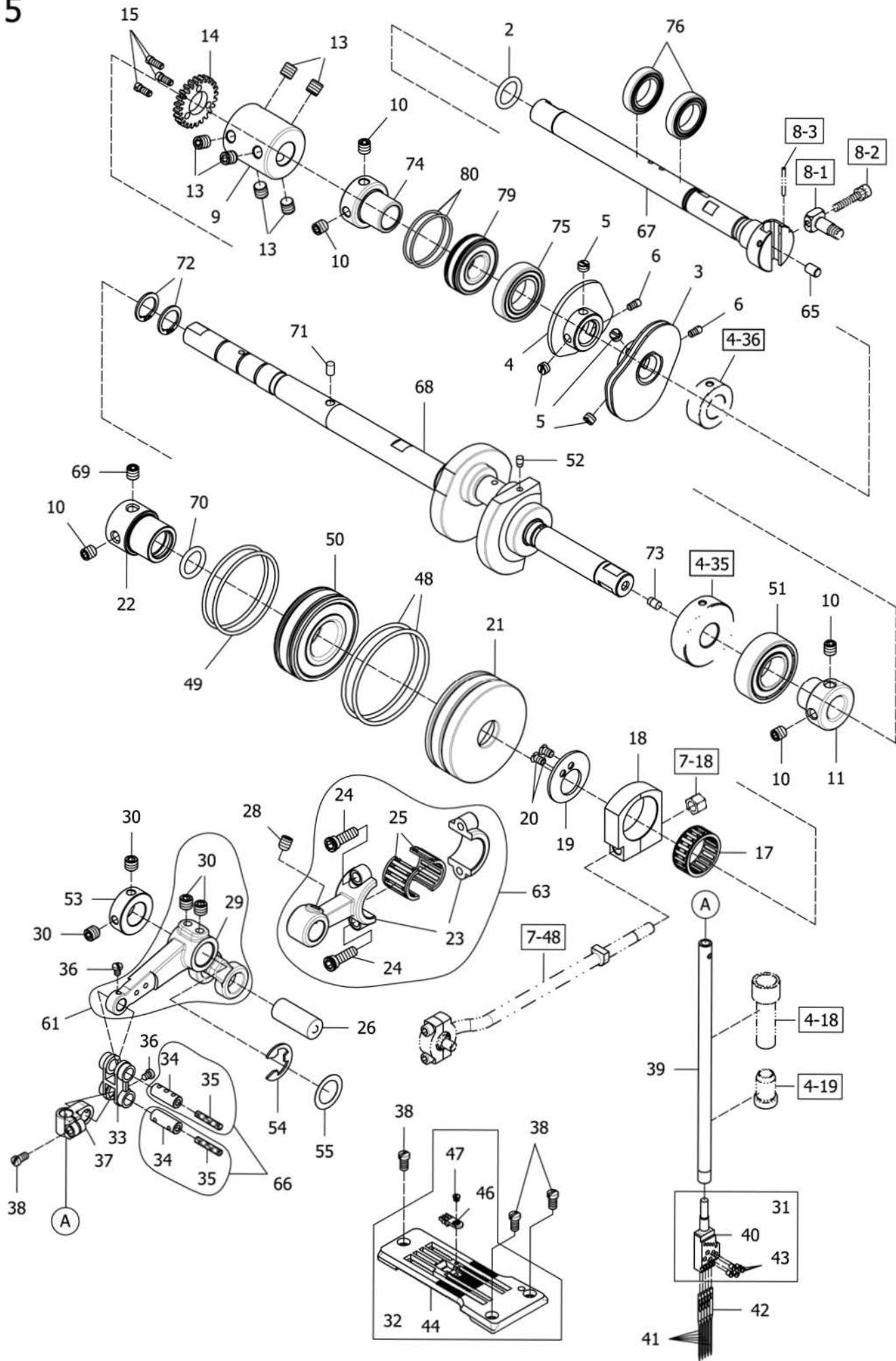
**MAIN SHAFT DRIVING MECHANISM**
