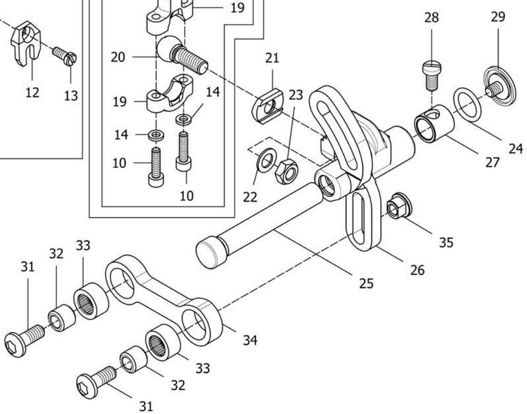
**FEED DRIVING CONTROL MECHANISM**
